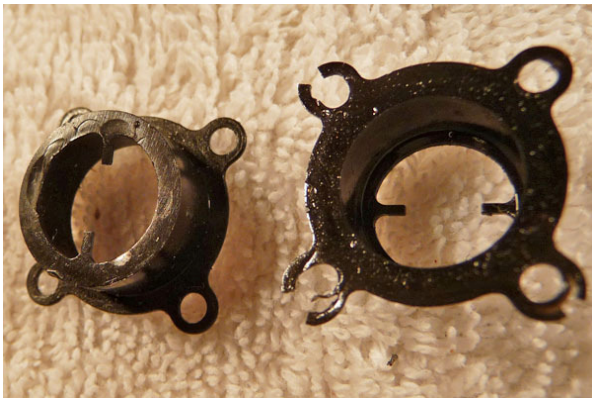
(L) excessive wear on top of reed retainer (R) cracked flange holes on reed retainer
