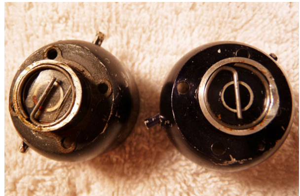
Black Widow tanks: note severe wear around reed retaining 'G-clip' area and reed seal venturi hole area.
