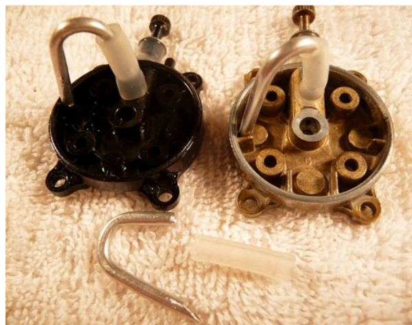
The replacement pick up tube is bent from 3/32" O.D. soft aluminium tubing & chamfered at the bottom to fit exactly. Silicone tubing attaches it to the tank back.
